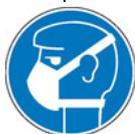
Wear respirator filter or breathing apparatus against vapours during thermal processing.
